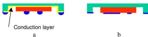
Fig. 3. a: Ball grid array (BGA) MOSFET package; b: large contact interconnect MOSFET package.
