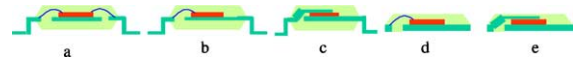
Fig. 1. Various types of SO-8 packages a: standard IC; b: standard power MOSFET; c: strap-bonded; d: leadless; e: strap-bonded with leadless.
